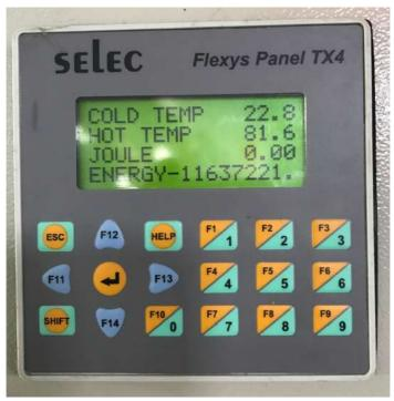
Figure 4: Solar hot air energy recorder
